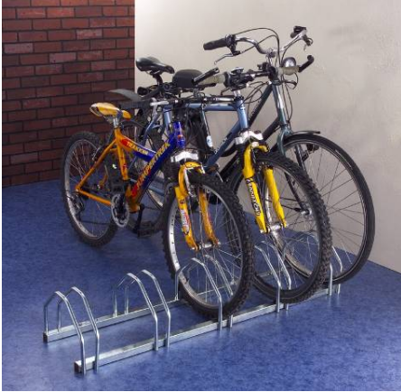
5 Cycle Rack. B131v Zinc plated steel construction. Designed to park 5 Bicycles. Length: 1340mm(300 mm centres) One piece – no assembly required.
